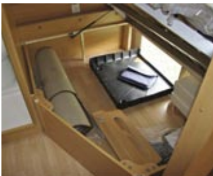
The protective hatch tray under the bed is useful but may hinder loading large items
