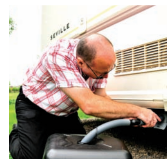
The waste drains are tucked under the skirt and tricky to access
