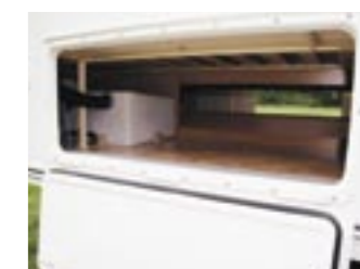
Through view, but the tank hinders the storage space
