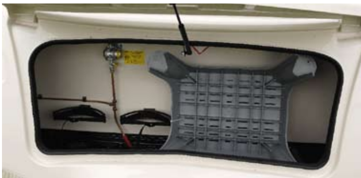
Front locker lid lifts on a gas strut to reveal plenty of storage space
