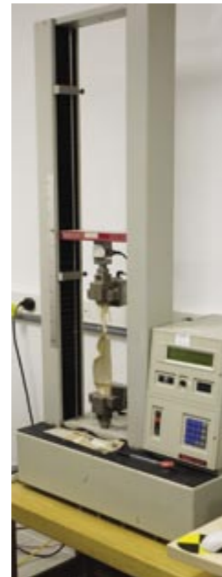
The strength of the upholstery fabric is tested to breaking point
