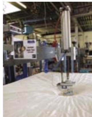
Durability testing on a caravan mattress
