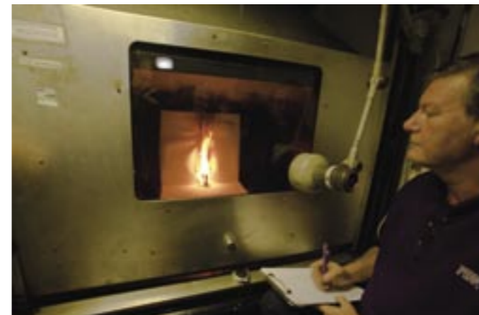
Upholstery foam is flame-tested to ensure it will not catch fire
