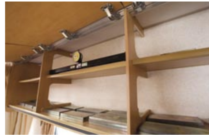
Wall cabinets are loaded to the limit to see if they will bow, then the weight is doubled, just to make sure
