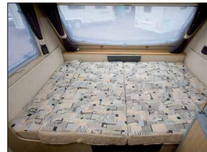
CLOCKWISE FROM ABOVE Pull-out slats make converting the lounge to a double bed simple. Seat boxes are carpeted but the lids stay up on their own. The fixed bed frame is rugged, but access to the inside is difficult
