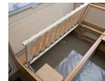
CLOCKWISE FROM ABOVE Pull-out slats make converting the lounge to a double bed simple. Seat boxes are carpeted but the lids stay up on their own. The fixed bed frame is rugged, but access to the inside is difficult
