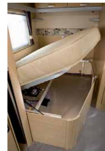
CLOCKWISE FROM ABOVE Pull-out slats make converting the lounge to a double bed simple. Seat boxes are carpeted but the lids stay up on their own. The fixed bed frame is rugged, but access to the inside is difficult
