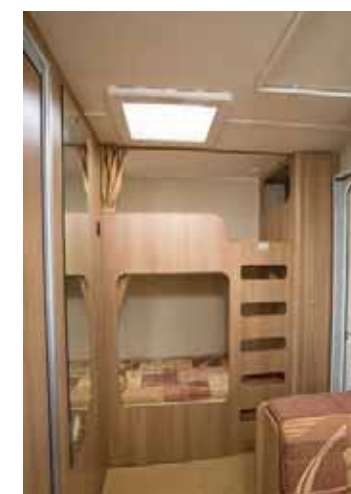
Rear bunk's fixed ladder restricts lower bunk access, but no stowing
